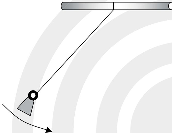
To make your pendulum, tie a string to a weight. Tie the other end of the string to something it can swing from. Learn what can change the time it takes to make one complete swing. Use a stopwatch to time one swing. Or, you can time ten swings and divide that number by ten.
