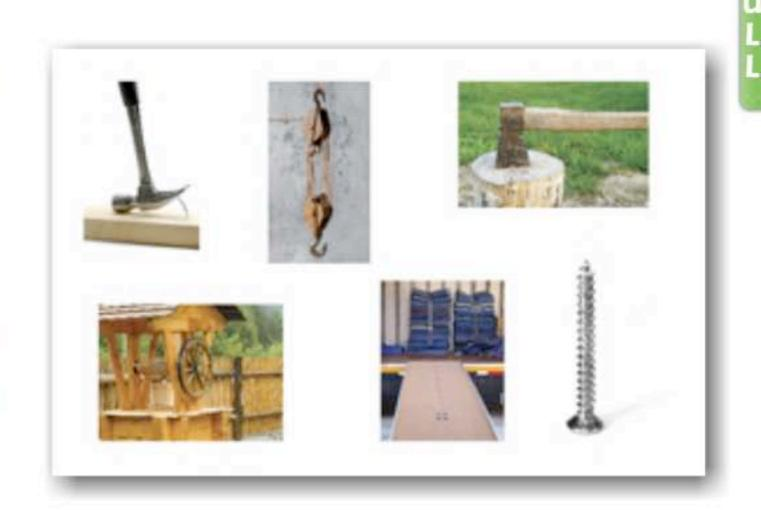
There are six kinds of simple machines: lever, wheel & axle, pulley, inclined plane, wedge, and screw. Look at the pictures of the six simple machines. It's easy to see how most of these work and how they change the force. We will look at each of these machines later on.
