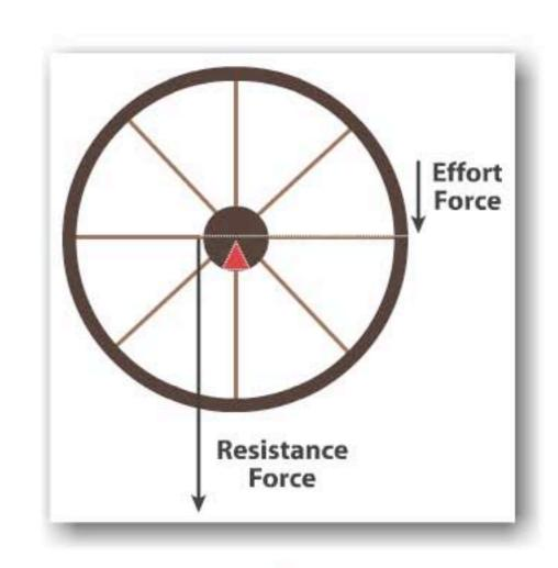
Pushing or pulling on the **wheel** turns the **axle**. The axle doesn't move as far as the wheel but it exerts a large resistance force.
