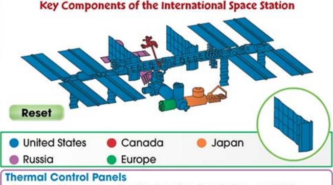
Allows heat to escape the ISS, keeping the station cool. This cooling system acts similar to the one used in a car radiator.
